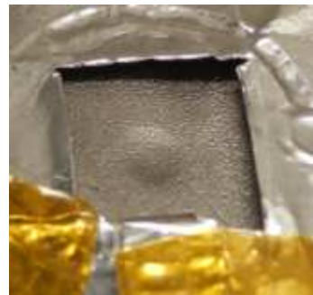
Figure 3 : Electrode achieved using spray-gun deposition method
